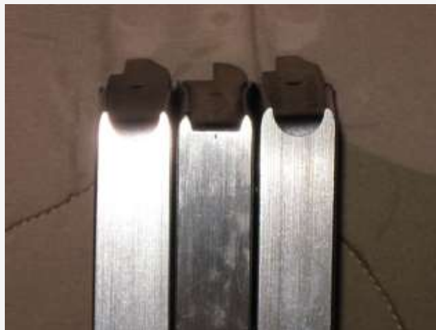
Standard 1911 magazine between two Sure Fire™ magazines, showing the rounded notch
