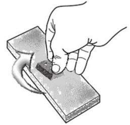
**IMPORTANT!** Push or tap only on the base of the dovetail otherwise damage may result.
